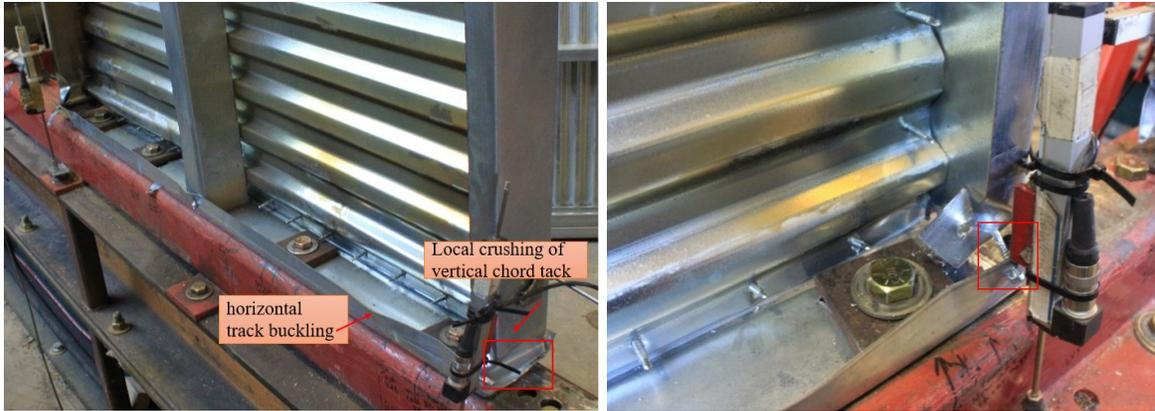
(b) Local crushing of vertical chord tack and horizontal track buckling; (c) Screw pull-out
