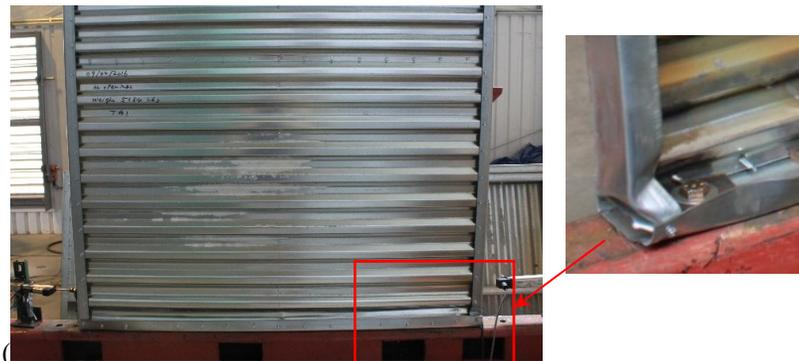
(a) Deformations after the loading process
